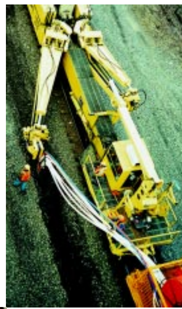
Our Railroad Mounted Cable Plow can operate from either side of the car with increased reach of plow arms.
